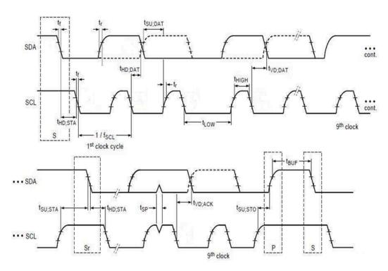
Figure 5: ZED-F9P-04B I2C peripheral specification
