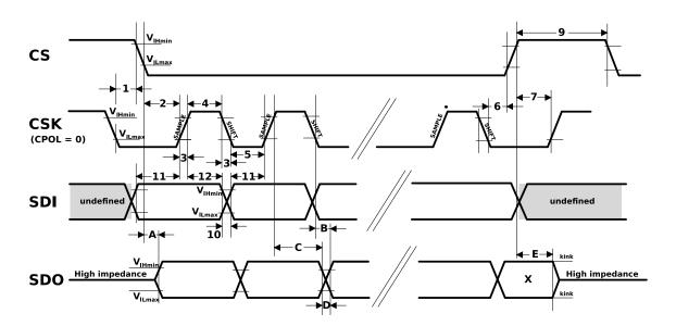
Figure 4: ZED-F9P-04B SPI specification mode 1: CPHA=0 SCK = 5.33 MHz
